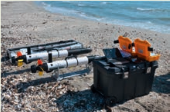
Pictures 3 and 4 — Sonar instruments used for marine cartography
