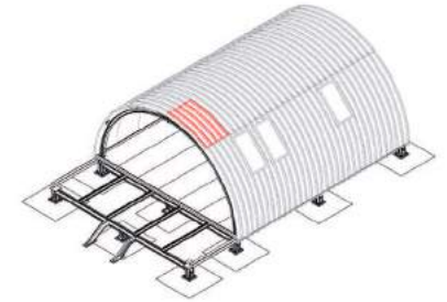
16. Polycarbonate corrugate sheet for ventilation
