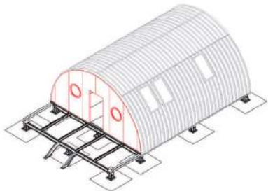
21. External wall in sandwich panels
