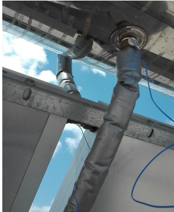
Figure 4.3: Thermocouple placement during natural circulation system check.
